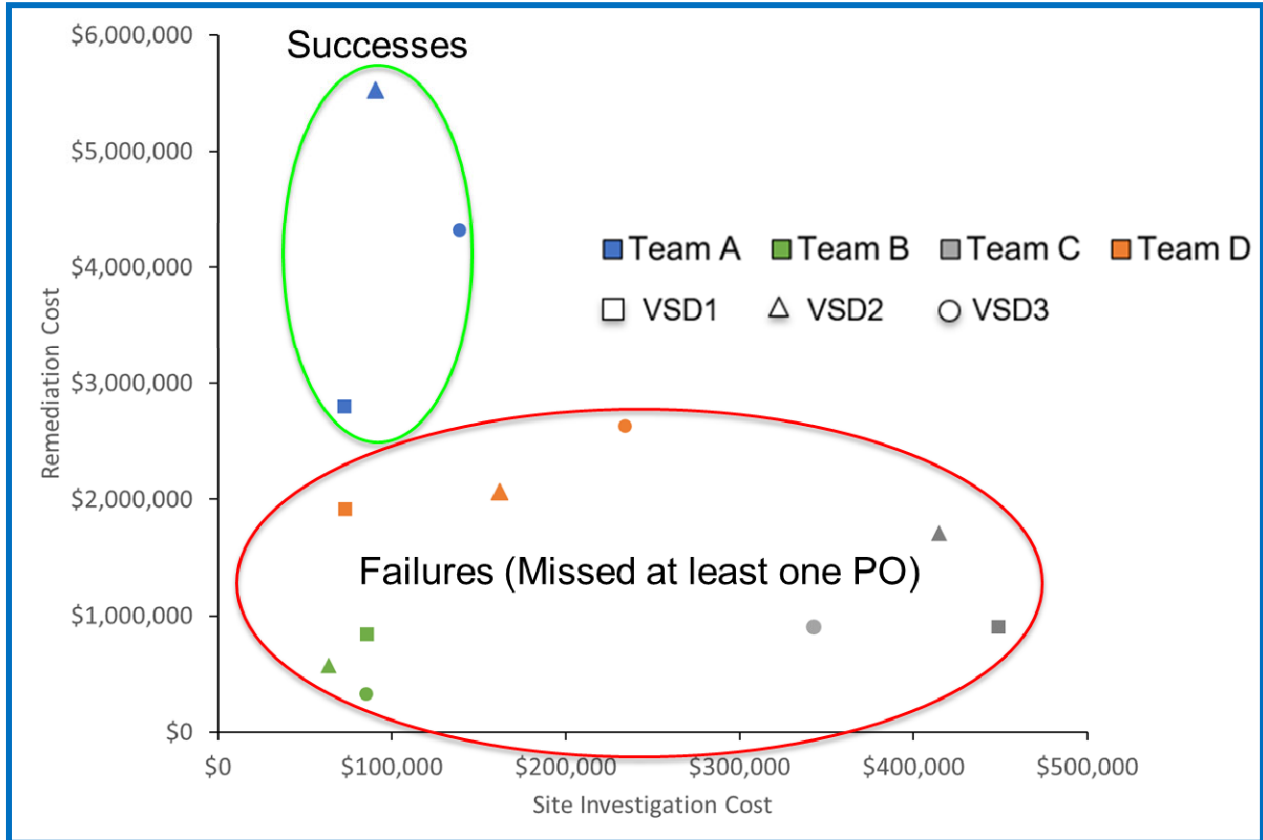
Figure ES – 6: Site investigation cost vs. remediation cost correlated to remediation success and failure
