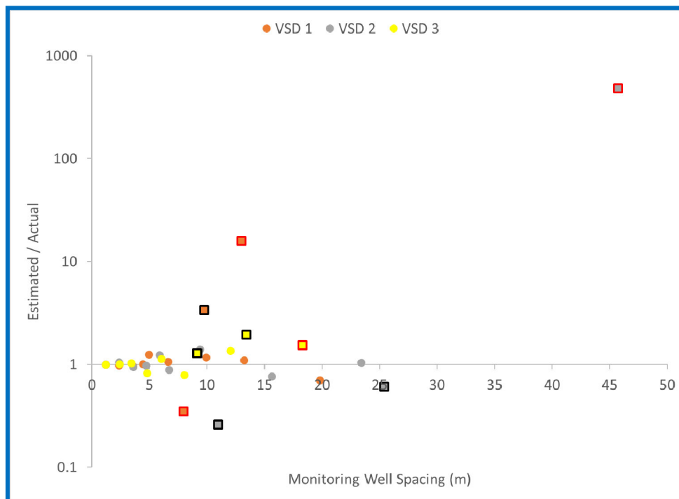
Figure 6-19: Comparison of DM Teams mass discharge estimates (squares) with expectations using a PFM approach (circles). Black outlined squares indicate where DM Teams used quantitative data. Red outlined squares indicate where DM Teams used qualitative data only.
