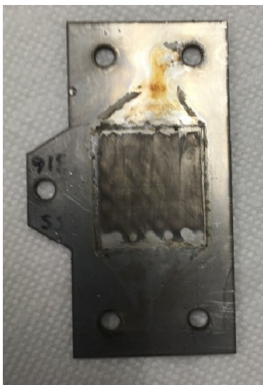
Figure 5.12. Corroded stainless steel cathode from the divided EC cell experiments.
