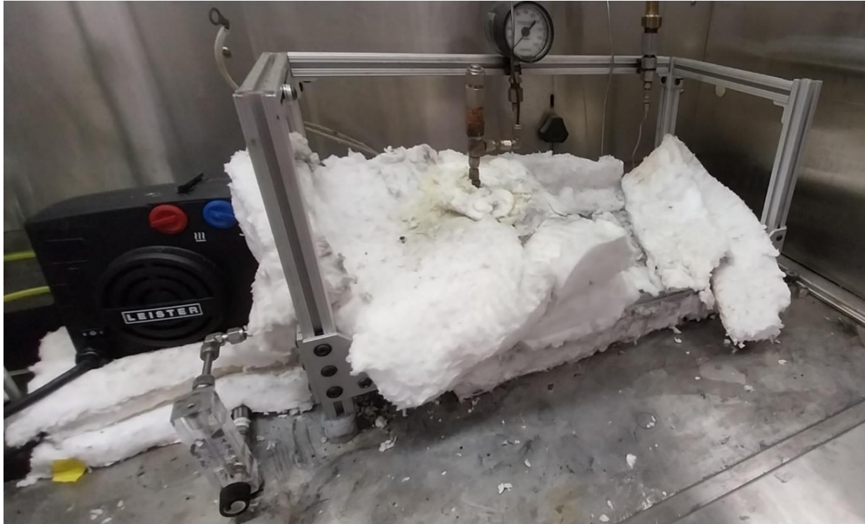
Figure 3: Experimental Reactor Equipment Heated using Hot Air Blower
