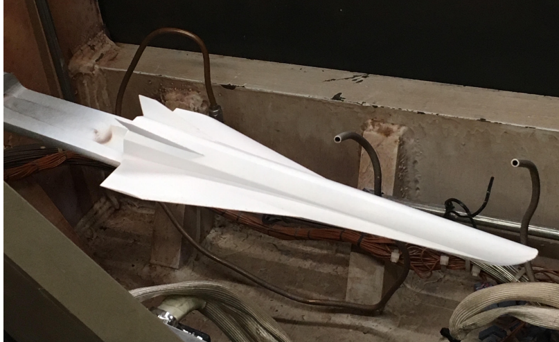
Figure 9: GHV Wind Tunnel Model with Thermal Sensitive Paint, from Sagerman et al. [31]
