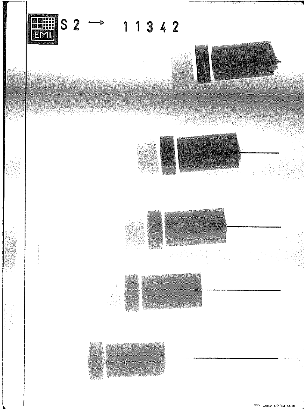
Figure A-15. X-ray picture for Exp. 11342: IT-SiC, v_p = 2.170 km/s.
