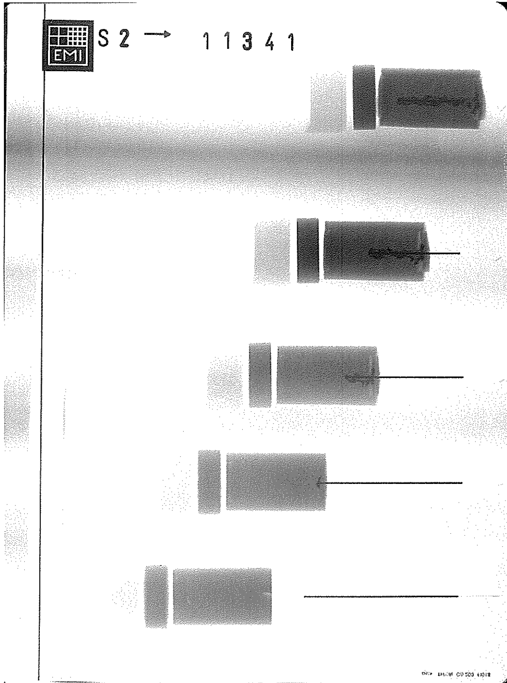
Figure A-1. X-ray picture for Exp. 11341: TS-SiC, v_p = 1.517 km/s.
