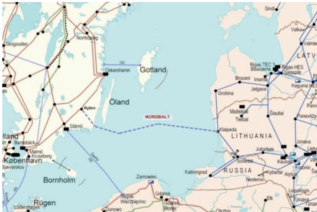
Figure 2.3. NordBalt Power Cable Location
