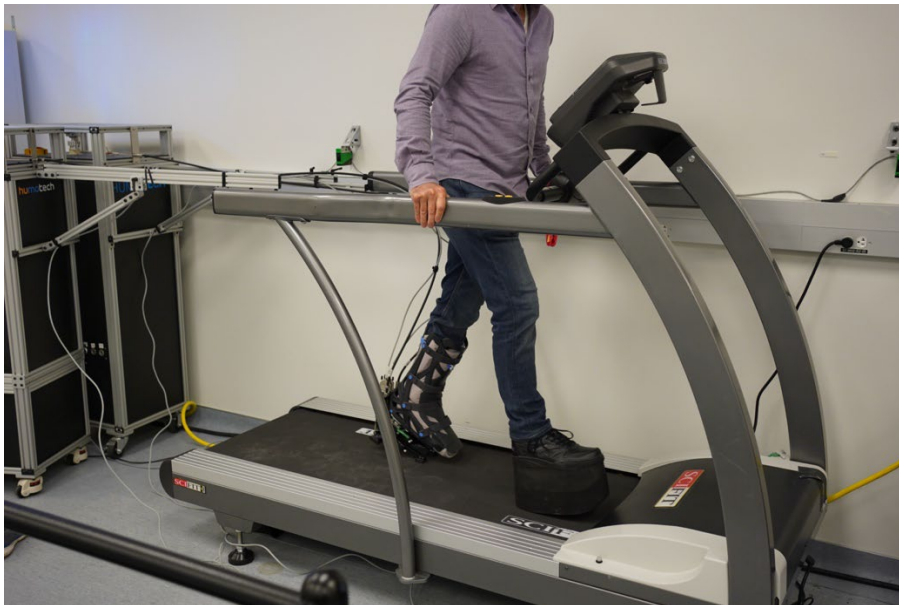
Figure 11. A team member wearing the PFE and a lift shoe while walking on the SciFit treadmill during a protocol practice run.
