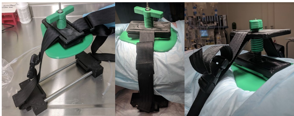
Figure 6. Initial prototype external compression system with sliding backplate, abdominal plate, and tourniquet style adjustment for compression depth.
