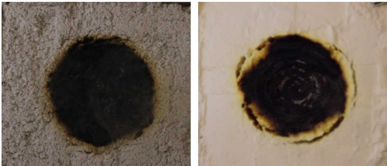
Figure 5.1.18: Images for burns with 100% cellulose (right) and 80% cellulose/20%lignin (left). Numerous large, dark cracks are visible outside the burned area in the 100% cellulose case.
