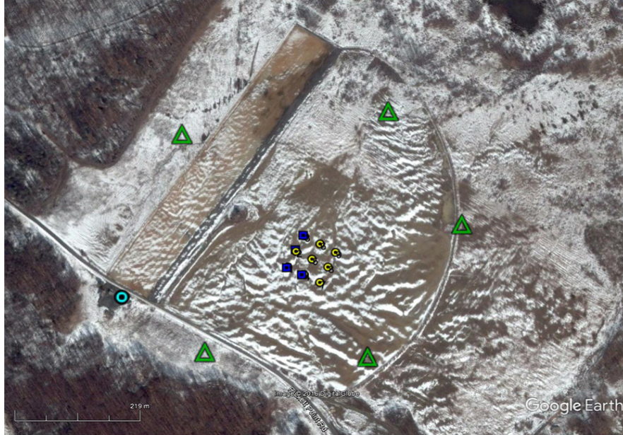
Figure 12. APG Impact Field with the Calibration Shots (Yellow Circles) and Located Positions (Blue Squares).
