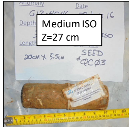
Figure 16. TOI in grid G12: (top) target 4048 and (bottom) target 4046. Both are medium ISOs at depth of 27 cm.
