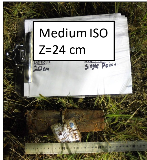
Figure 15. TOI in grid B12: target 2068, a medium ISO at depth of 24 cm.
