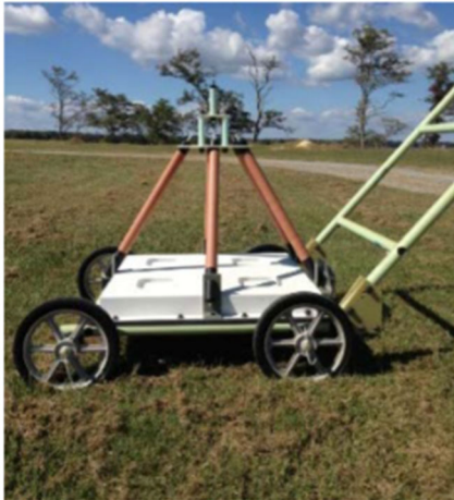
Figure 1. Left: Cued TEMTADS 2x2 array with GPS mount. Right: Sensor geometry showing four transmitters (solid black lines) and concentric 3-axis receivers. Photo credit: TEMTADS 2x2 user manual.
