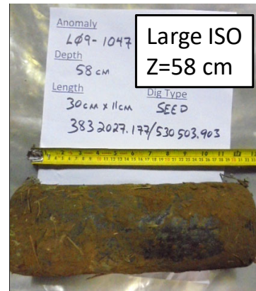
Figure 19. TOI in grid L09: (top) target 1043, a medium ISO at 52 cm depth; and (bottom) target 1047, a large ISO at depth of 58 cm.
