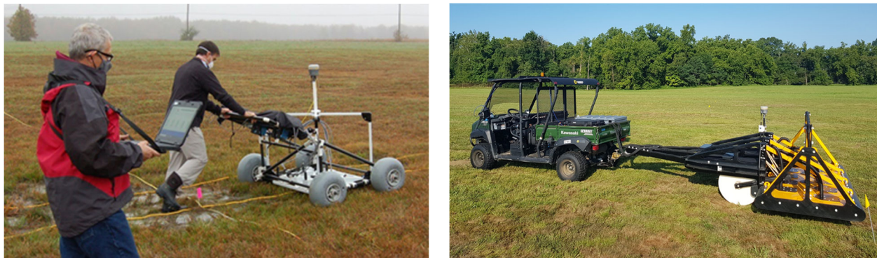
Figure 8. AGC Sensors Validated for One-pass Classification. Left: The APEX Sensor. Right: The UltraTEM Towed Array.
