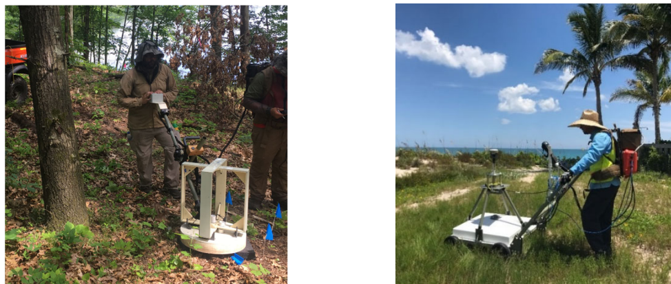
Figure 7. Examples of Validated AGC Sensors. Left: MPV (Shown in Cued Mode). Right: MetalMapper 2x2.
