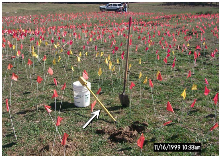
Figure 2. Detections from a “Mag and Flag” Survey Carried Out with a Schonstedt Passive Magnetometer.
