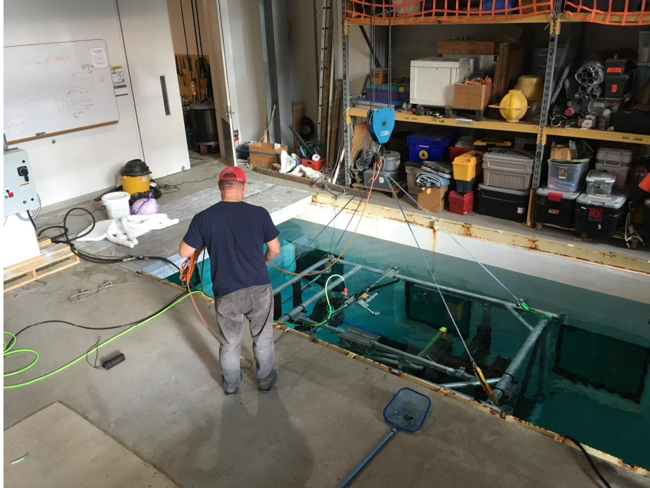
Figure 3. Test frame suspended in University of Washington School of Oceanography test tank. Hydraulic pressure unit (HPU) for operating the Schilling arm is just visible to left.
