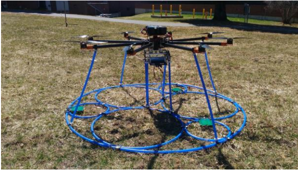
Figure 56: UAS EMI system: consists of four Tx coils. The radius of Tx-1 is 1.616 m, and radius of Tx2, Tx-3 and Tx-4 coils are 75 cm. It has high density polyethylene tubing, 3-D printed custom connectors and coils are threaded into tubes for protection, and contains nonmetallic parts.
