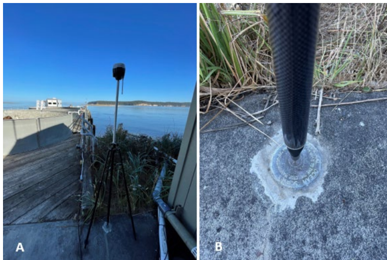
Figure 6. (A) Tripod-mounted RTK-GPS base station over the geodetic marker. (B) NGS geodetic marker on the PNNL-Sequim campus.
