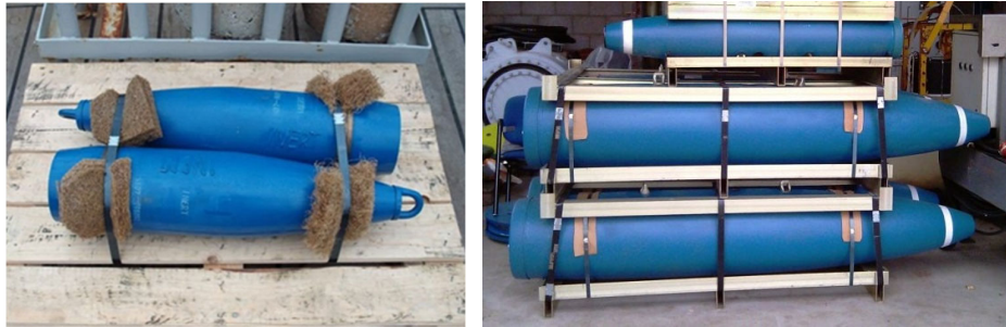
Figure 1-2: Example of UXO exercise objects; 155 mm shells (left) and 2000 lb concrete filled bombs (right).
