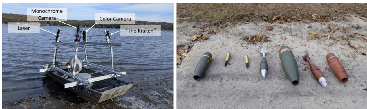
Figure 2. The Assembled Proof-of-Concept System (Left) and Replica Inert Munitions (Right)
