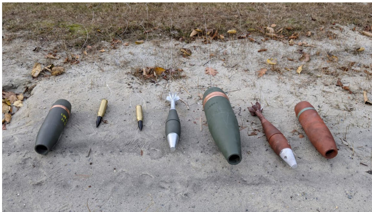
Figure 9. Inert Replica Munitions, from Left to Right: 105mm Artillery Projectile, 2x 25mm Bushmaster Rounds, 81mm Mortar, 155mm Artillery Projectile, 81mm Mortar (UXO), 105mm Artillery Projectile (UXO).
