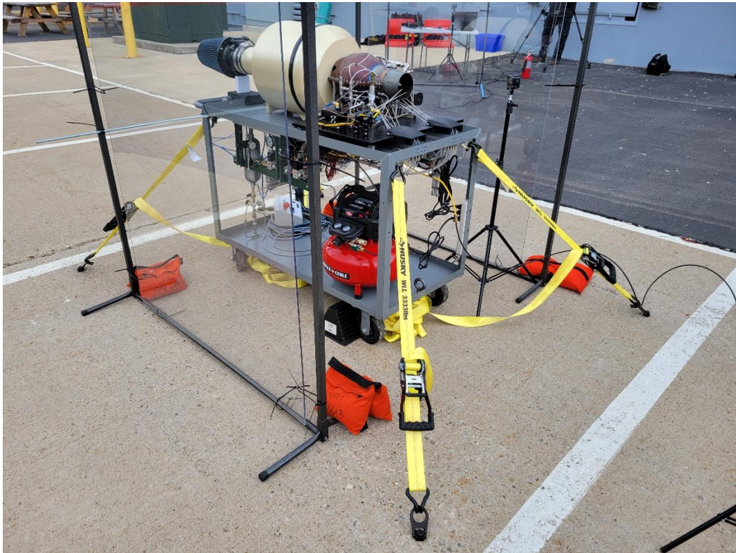
Figure 19. Mobile Engine Test Stand Setup
