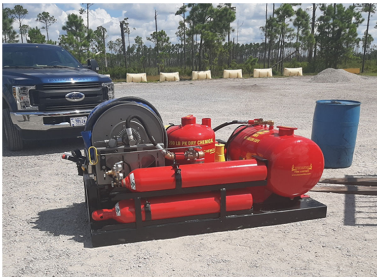
Figure 6. Dual-Agent CAF Skid for 315-ft 2 Fire Tests
