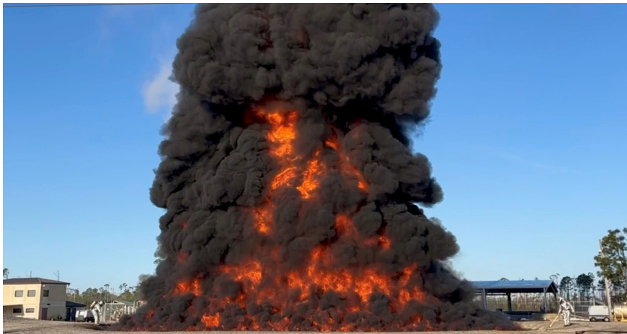
Figure 7. Manual Ignition of 1000 Gallon Aviation Fuel. Research and Test Pool-II (Silver Flag Test Site, Tyndall AFB)
