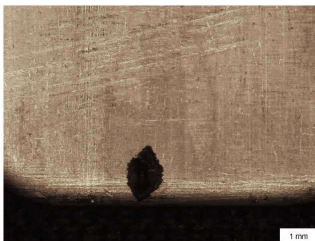
Figure E-21. Crevice Attack Observed on Stainless Steel Sample 70, Foam #8
