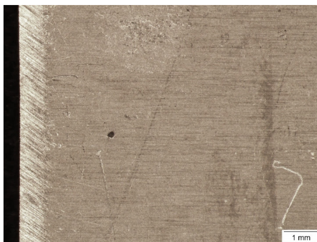
Figure E-19. Isolated Pitting Observed on Stainless Steel sample 25, Foam #4
