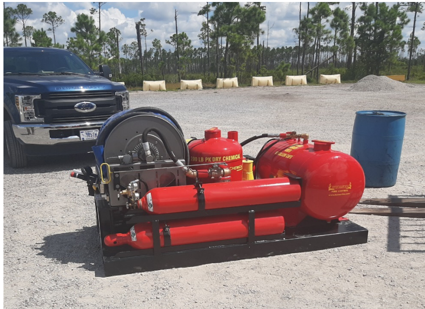
Figure 7. Dual-Agent CAF Skid for 315-ft 2 Fire Testing
