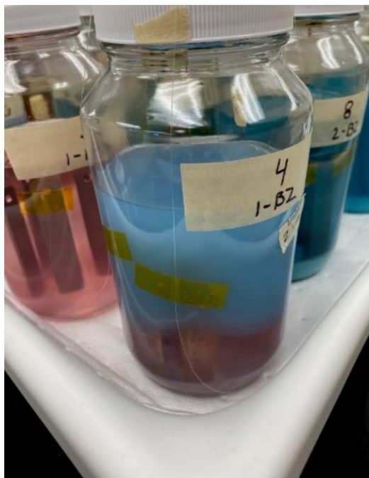
Figure E-24. Foam #1 Exhibiting a Phase Separation into a Milky Blue Low-density Phase and the Native Pink Foam Solution.
