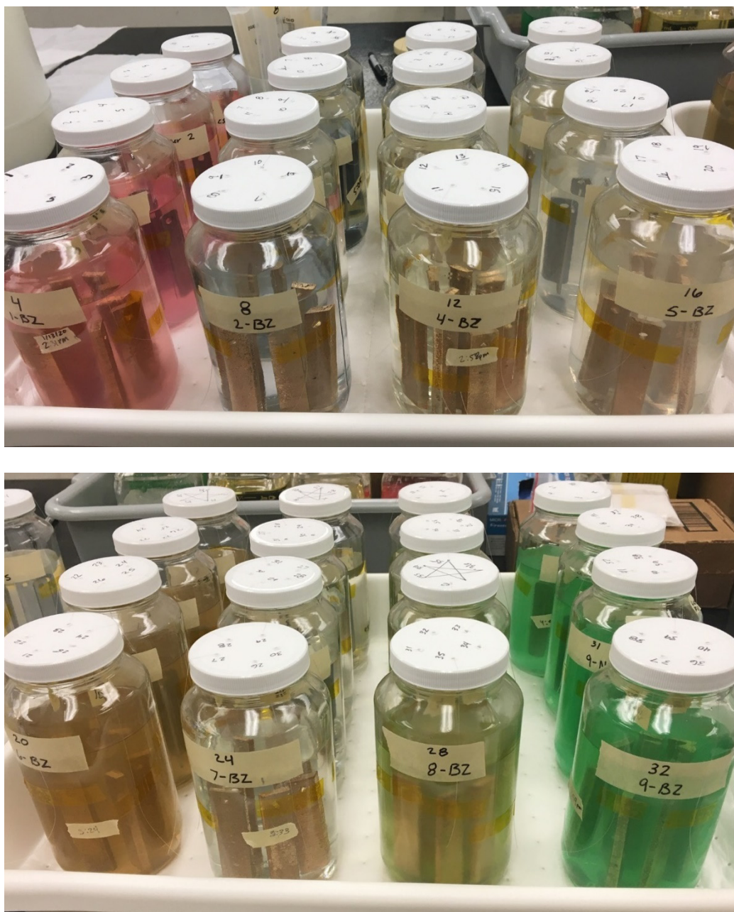
Figure E-2. AFFF Exposure Containment Cells – General Corrosion Rate Study.
