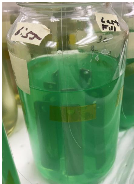
Figure E-1. Example Exposure Depicting the Material Coupons Suspended in Solution.
