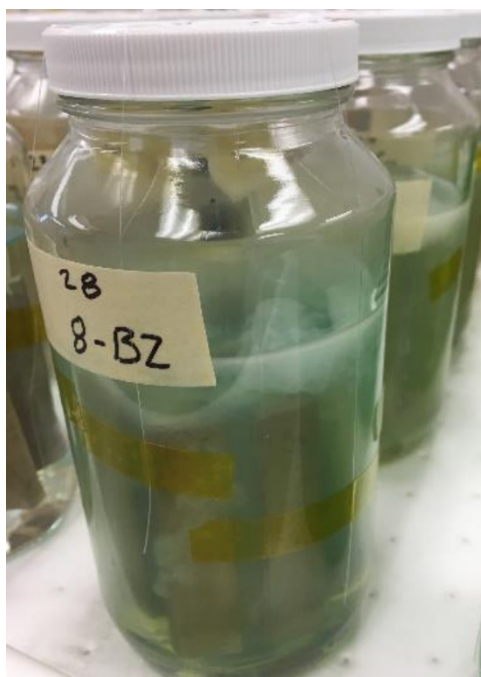
Figure E-25. Foam #8 Example of Coagulant Collecting at the Solution Surface and Along the Length of the C90500 Specimens.
