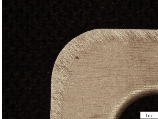
Figure E-22. Isolated Pitting Observed on Stainless Steel Sample 72, Foam #9
