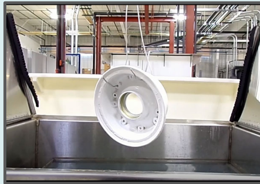
Step 1: The wheel is ready to be dispensed in the sonicator
