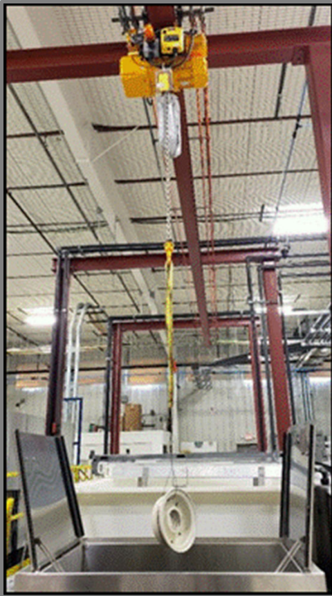
Set-up for suspending the wheel in the sonicator
