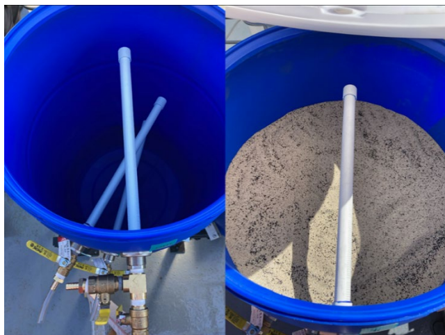
Figure 8: Internal view of reactors before and after filling with the GAC/sand mixture.
