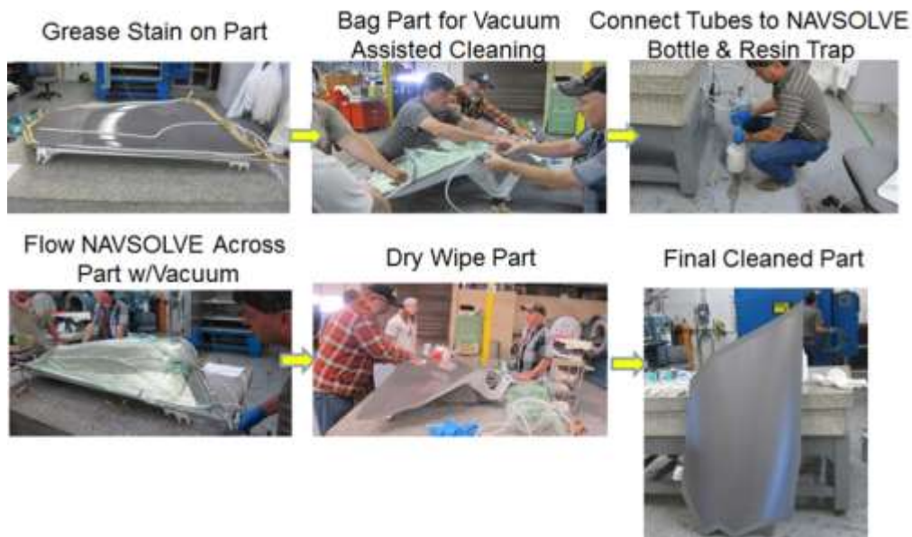
Figure 5. Steps in vacuum assisted cleaning demonstration with NAVSOLVE™ at Hill AFB
