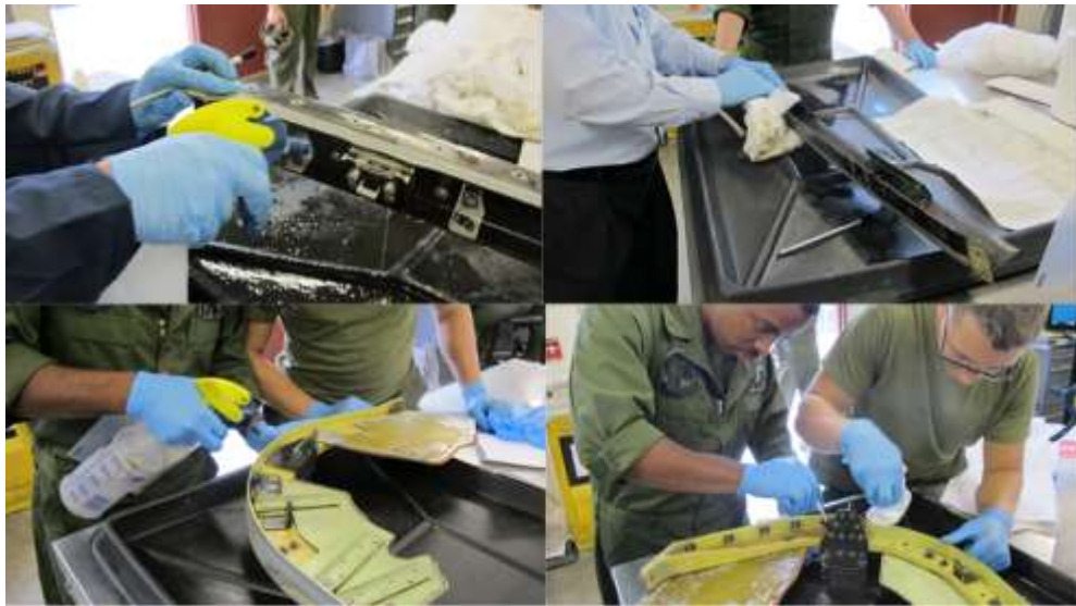
Figure 4. Cleaning demonstration on V-22 composite parts at MCB Camp Pendleton
