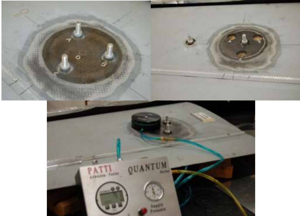
Figure 40. PATTI test set-up; pull stubs bonded, and OML skin/core removed around stub prior to testing
