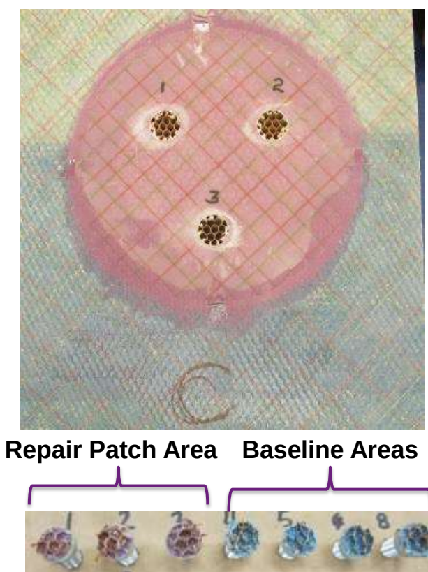
Figure 55. PATTI results for NAVSOLVE™ cleaned, bonded repair patch
