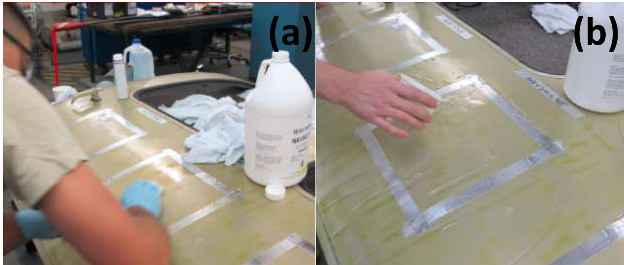
Figure 58. Section 2 (NAVSOLVE™): (a) hand wipe cleaning followed by (b) water break test
