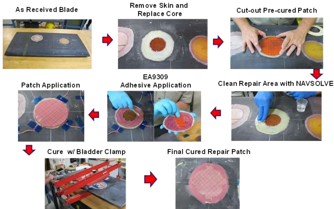
Figure 6. Steps in bonded patch repair of helicopter composite blade section using bladder clamp
