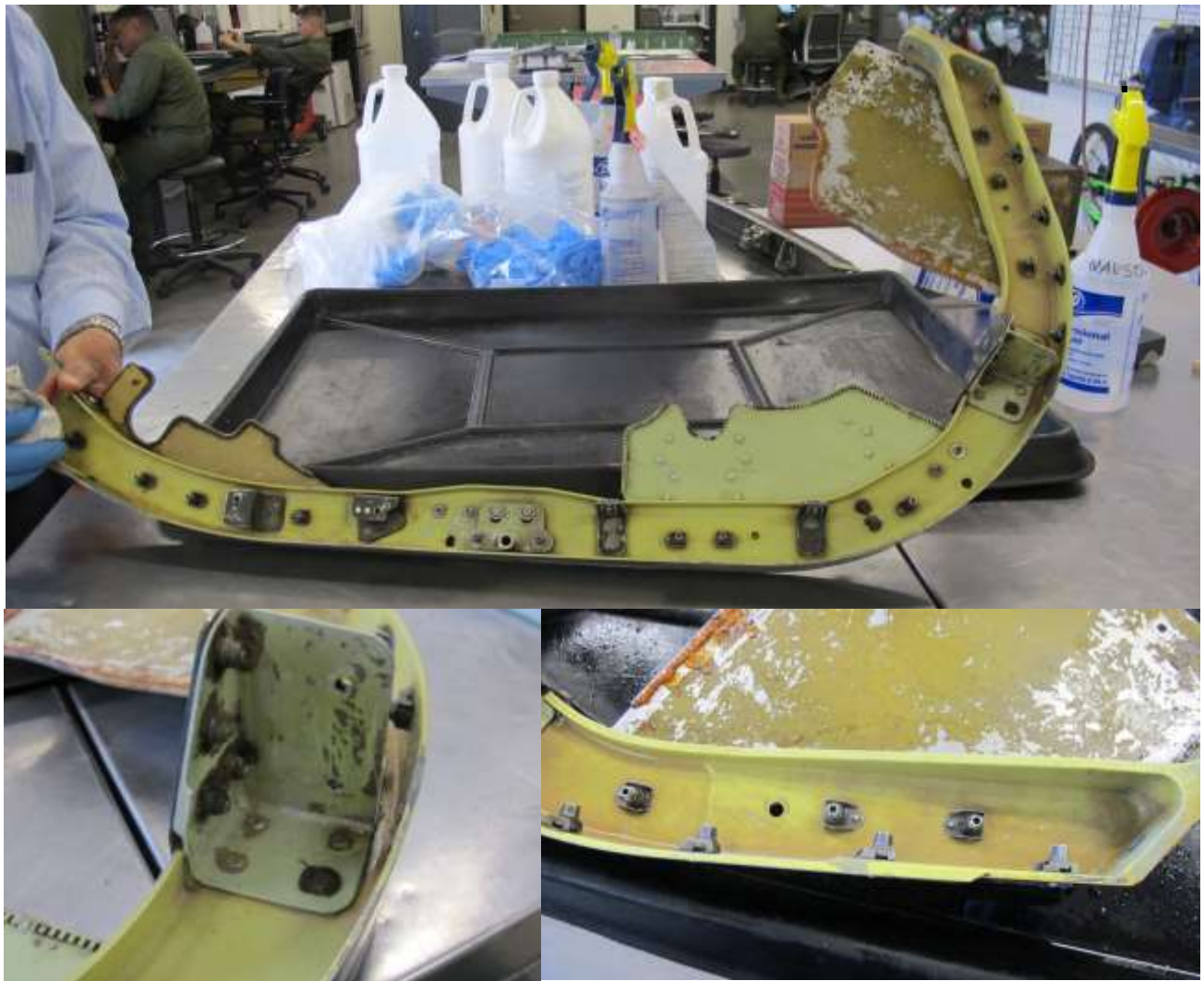
Figure 64. Final primed V-22 composite demonstration part cleaned with NAVSOLVE™
