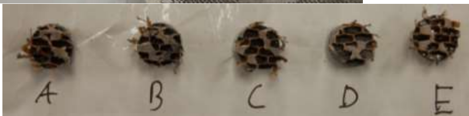
Figure 41. Pull out results of PATTI test on UAV wing section
