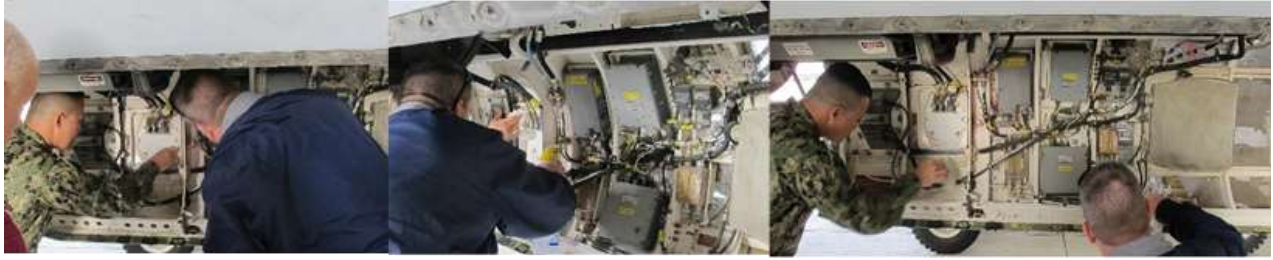
Figure 3. Cleaning demonstration with NAVSOLVE™ of F/A-18 bay on flight-line at NAS Lemoore
