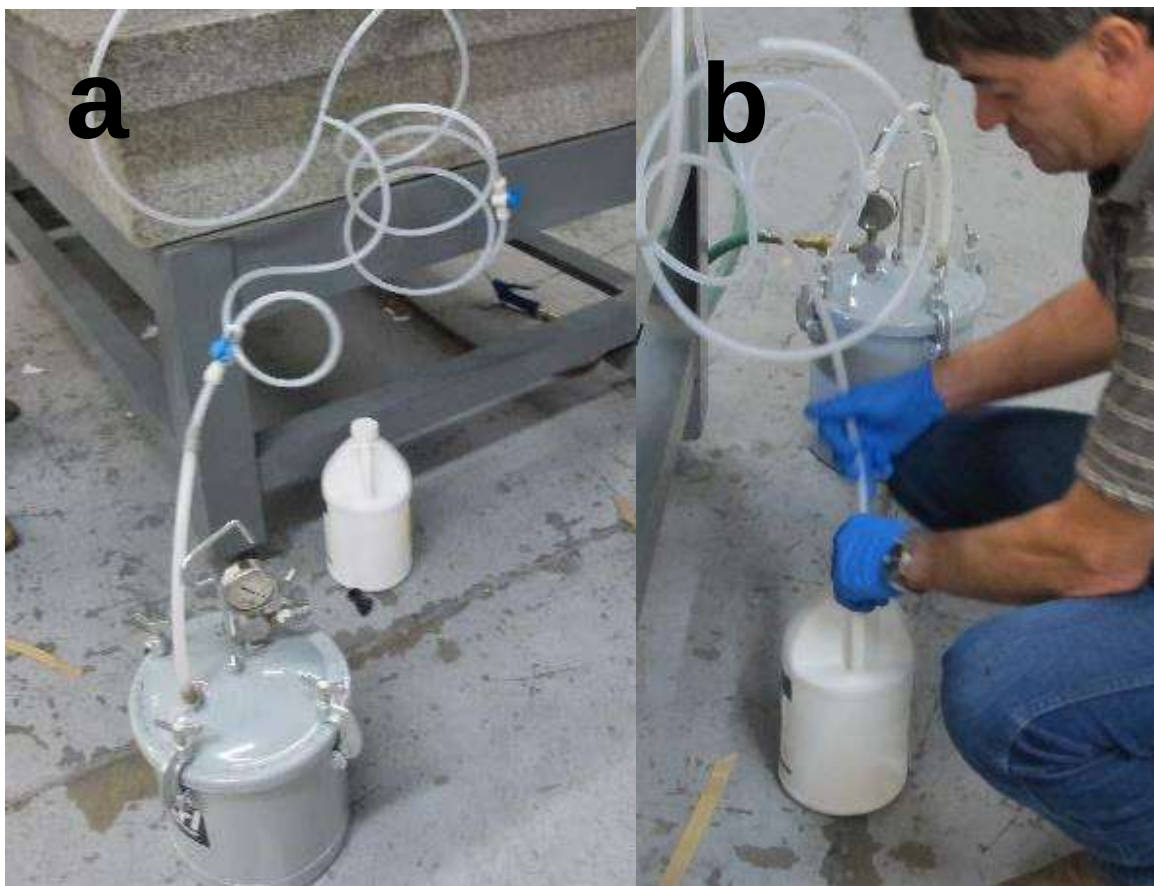
Figure 48. Tubing connection to a) VARTM resin trap and b) jug of NAVSOLVE™ cleaner
