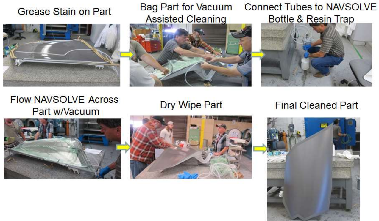
Figure 49. Steps in vacuum assisted cleaning demonstration with NAVSOLVE™ at Hill AFB
