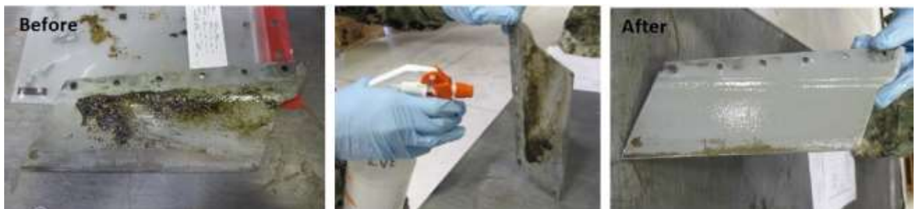
Figure 66. Cleaning demonstration with NAVSOLVE™ on F/A-18 part contaminated with heavy grease
