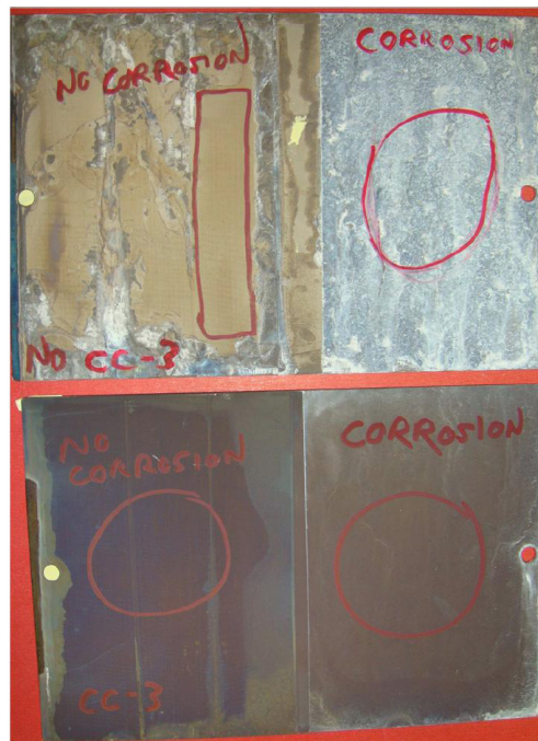
Figure 6. Corroded and Un-corroded areas of LHE Zn-Ni Panes CC-3 (bottom) and NCC-3 (top) after Four Weeks in ASTM B117 Salt Spray
