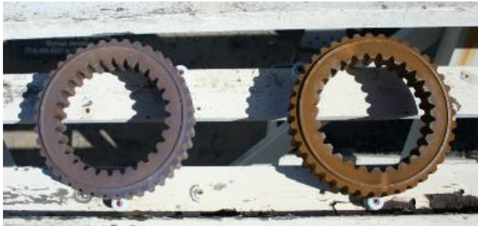
Figure 19. Corrosion Test Subjects on Installation (11/3/2014)
