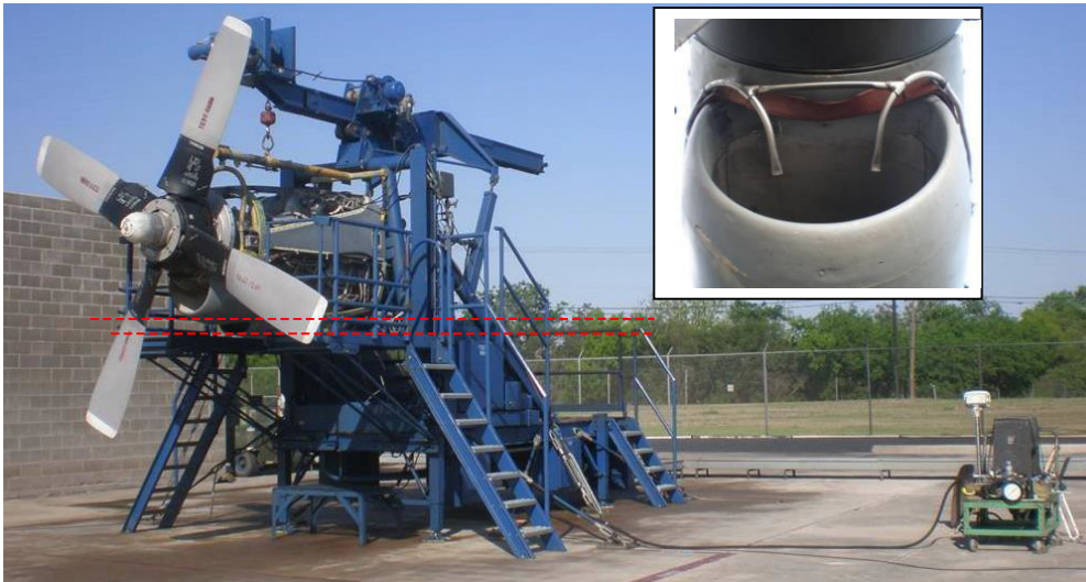
Figure 11: Engine Sand Ingestion Set-Up METS at SASAI
