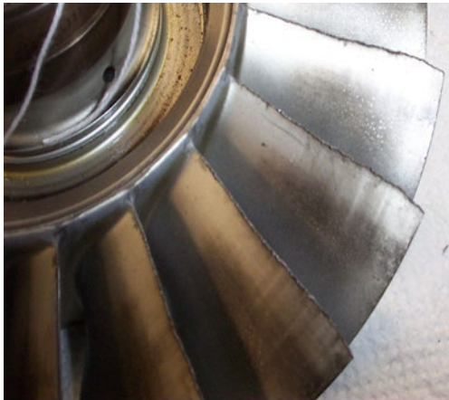
Figure 23: T700 with Sharp LE 1st Stage Blisk Airfoils Establishing LE Curl
