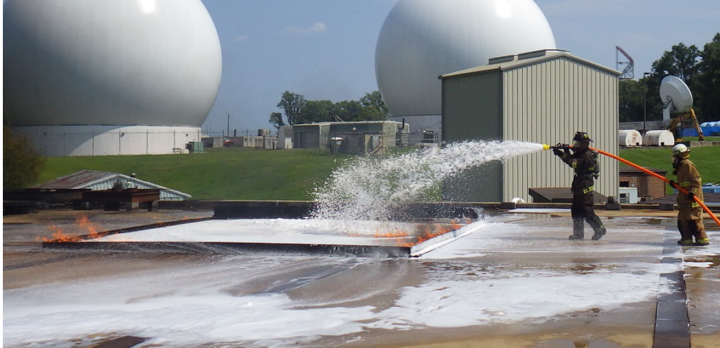
Figure 7.7. 30 gpm Nozzle with Foam Tube at 5 Degree Spray Pattern
