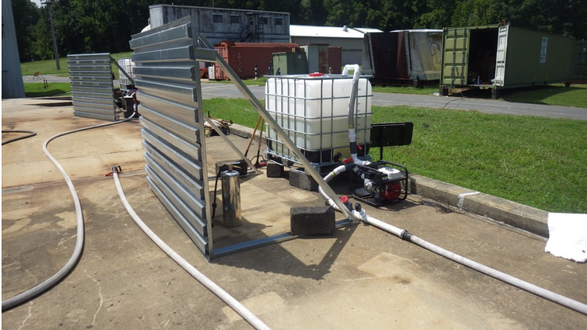
Figure 7.4. Primary and Backup Manual Firefighting Systems
