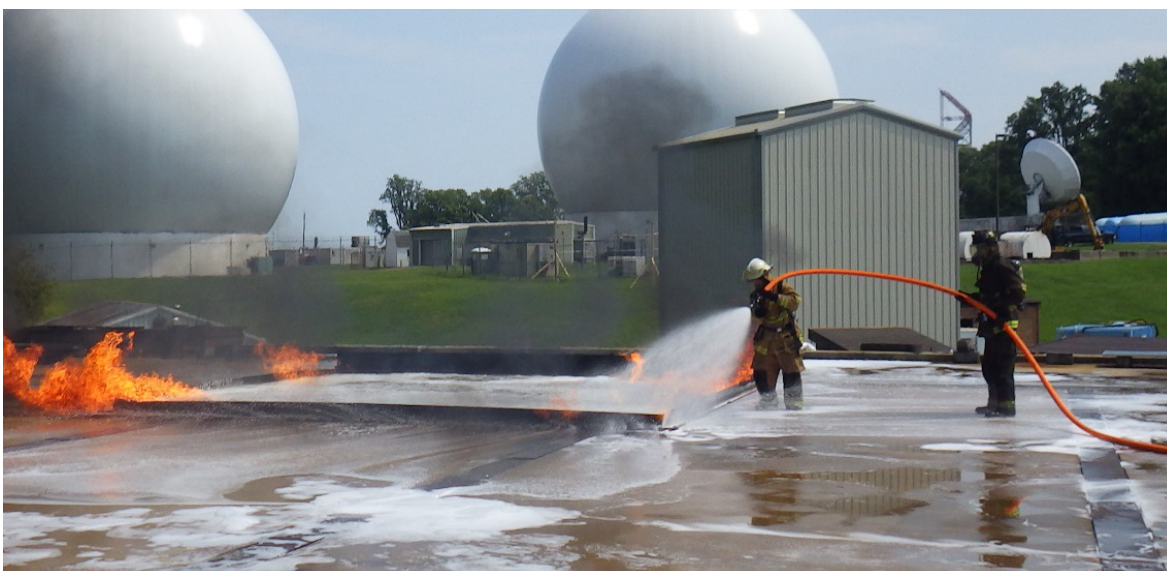
Figure 7.6. Standard 30 gpm Nozzle at 15 Degree Spray Pattern
