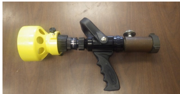
Figure 7.5. 30 gpm Nozzle with and without the Foam Tube Adapter
