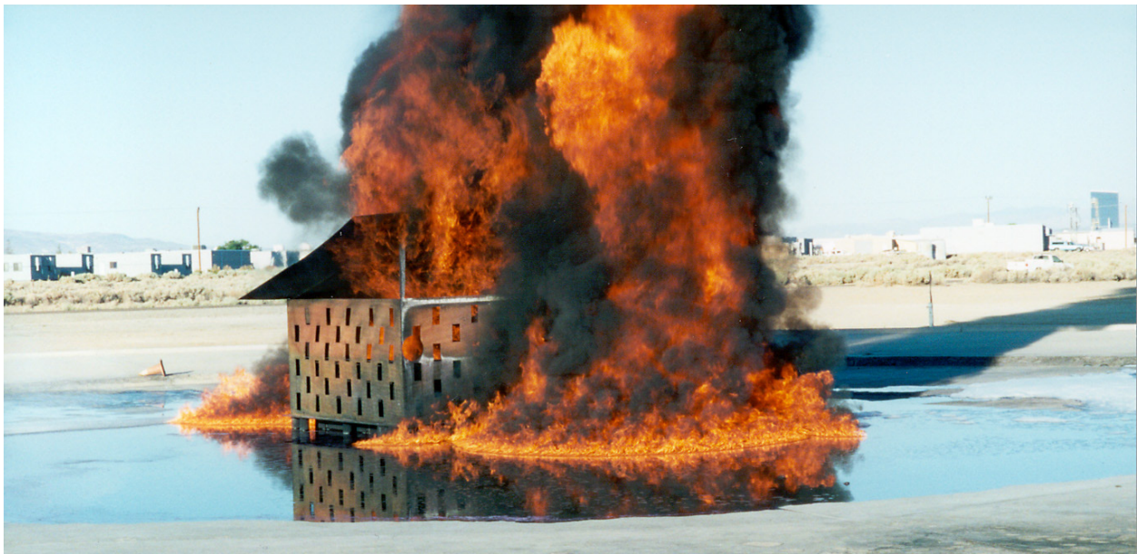
Figure 11.3. Legacy Debris Pile Constructed with Steel Walls and Roof
