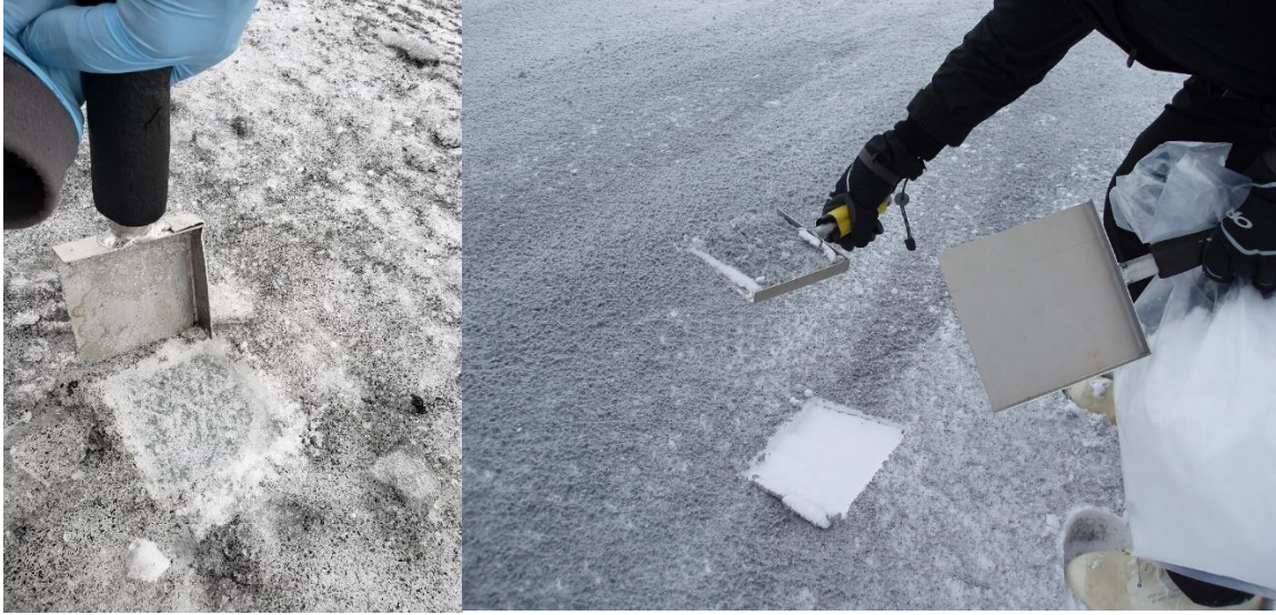
Figure E4. Left: outline chisel sampling on hard snow; right: one-motion scoop sampling on soft snow (note: larger 20-cm scoop pictured).
