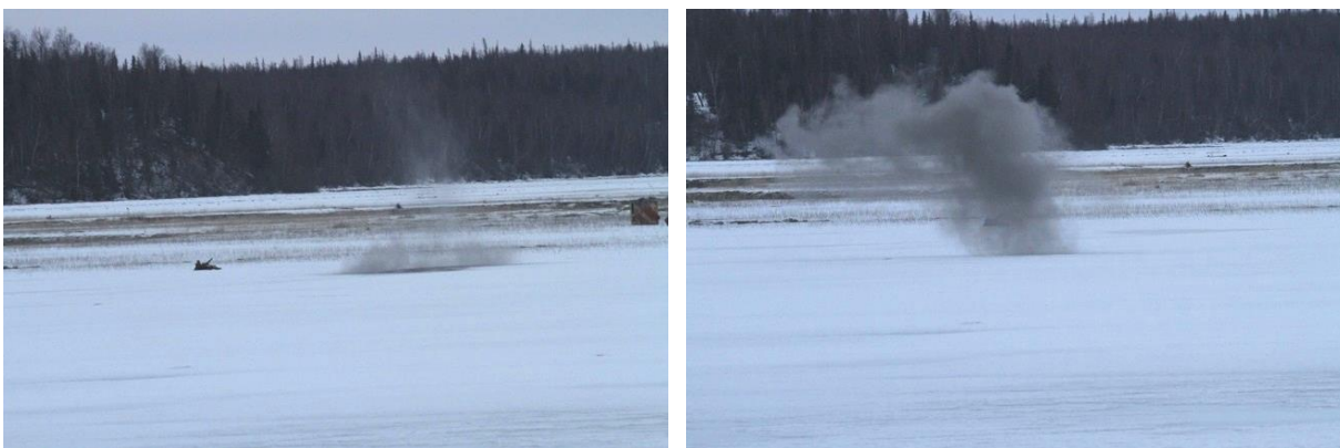
Figure 33. Residue and soot clouds immediately after detonation of a 60 mm munition (M720A2) using the IMP (left) and PRX (right) settings on the M734A1 multi-option fuze.
