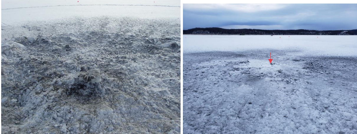
Figure 25. Examples of plume centers from command-detonation (left) and live-fire (right) tests of M720A2 60 mm IMX-104 mortar cartridges. Red arrow indicates the estimated impact point.
