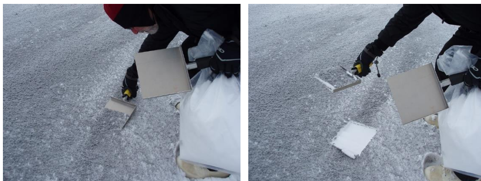
Figure 14. Example of complete residue collection with a 2.5-cm deep snow scoop (20-cm x 20-cm scoops pictured).
