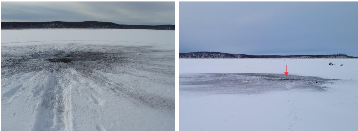
Figure 30. Examples of plume centers from command detonation tests of M821A3 (left) and live-fire tests of M889A4 (right) 81 mm IMX-104 mortar cartridges. Red arrow indicates the estimated impact point.
