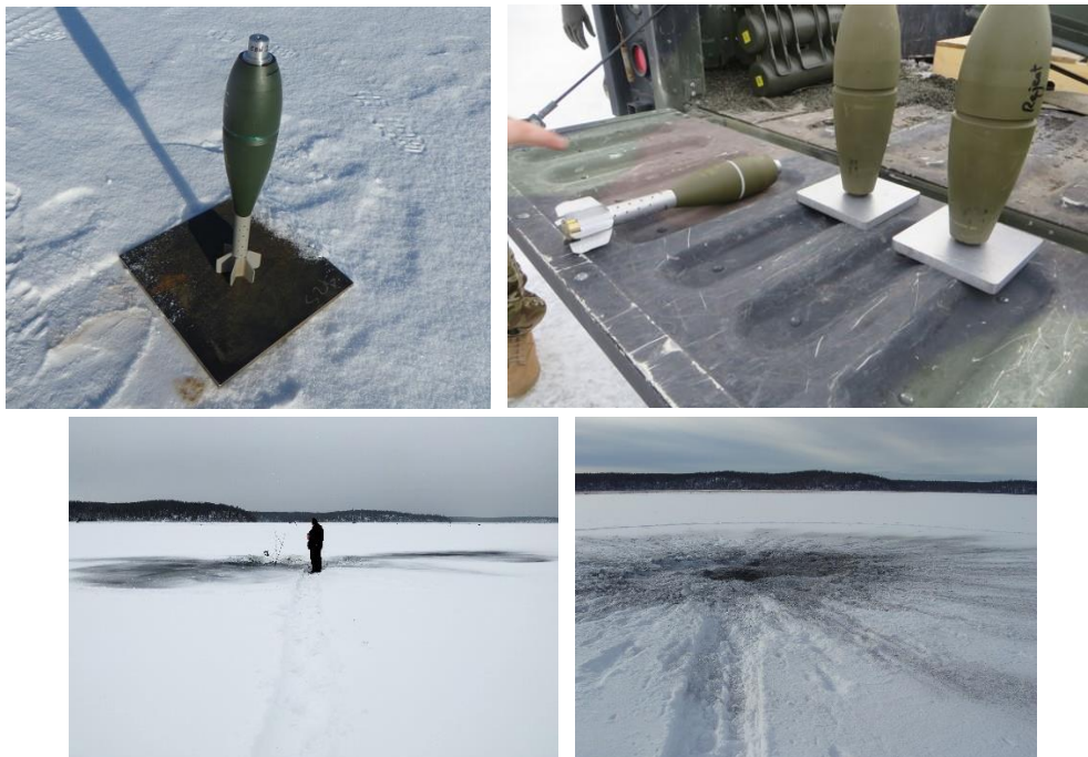
Figure E1. Clockwise from top left: an 81 mm cartridge with tailfin nose-up with CFS on a steel plate; a 60 mm mortar cartridge with tailfin and two 81 mm mortar round bodies mounted on aluminum support plates; symmetric dispersion of residue and soot from an 81 mm mortar cartridge with CFS in vertical position; and asymmetric dispersion of residue and soot from a horizontally placed 155 mm practice round with AFS.
