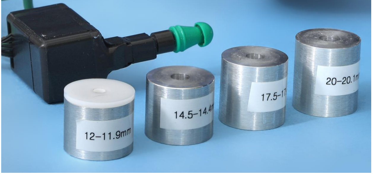
Figure 3. Aluminum Cavities used for Probe Calibration.
