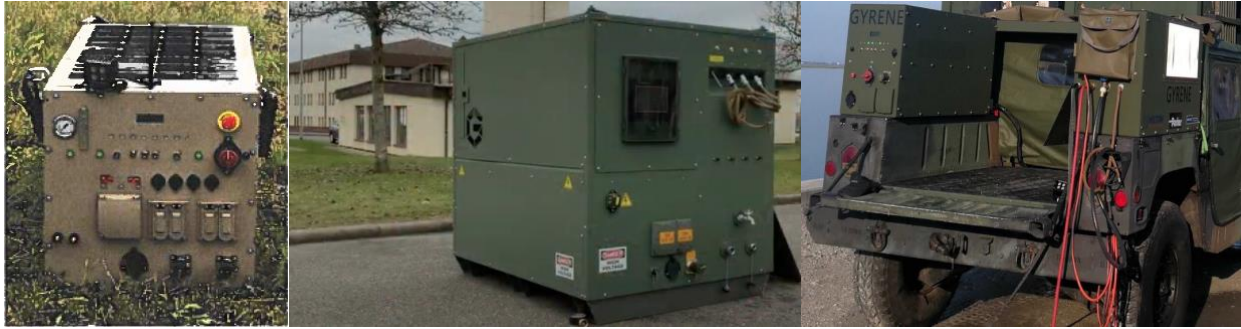
Figure 2. Gyrene Engineering Management's Mangrove. An expeditionary, modular, water and energy harvesting system designed for fire-team to platoon-sized operations. Note: Illustrations from left to right, P-1A stand-alone, P-3A skid-mounted, and P-3B vehicle-integrated systems.
