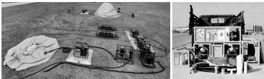
Figure 5. Lightweight Water Purification System. (Left to right) off-loaded assembled system and disassembled components near a truck. Reprinted from MCRP 3-40D.14, Water Support Operations, fig. A-4 and fig 4-9.
