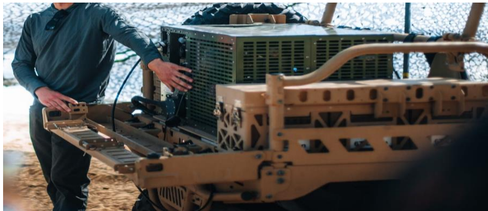
Figure 1. Mounted Atmospheric Water Generator. Photo credit, Corporal Patrick King. (Adapted from Kelsey D. Atherton, “Make Drinking Water from Thin Air,” Popular Science , 29 November 2022, https://www.popsci.com/technology/marine-corps-atmospheric-portable-water-sustainment-unit/ .)
