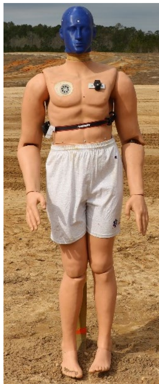
Figure 2. Instrumented manikin: example of torso and head combination.
