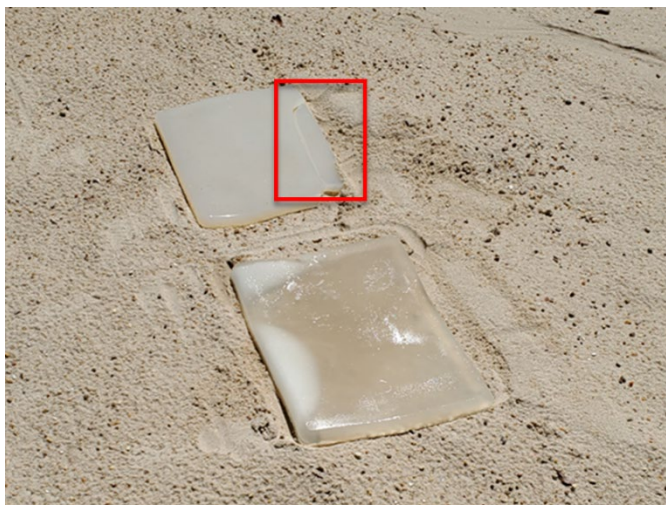
Figure 12. Bulk hydrogel used in field studies to observe thermal signatures of gel matrices versus control: simple agar hydrogel with red box showing small area of mechanical instability immediately upon environmental exposure ( top ) and clear bulk alginate-LiCl hydrogel reported herein ( bottom ).
