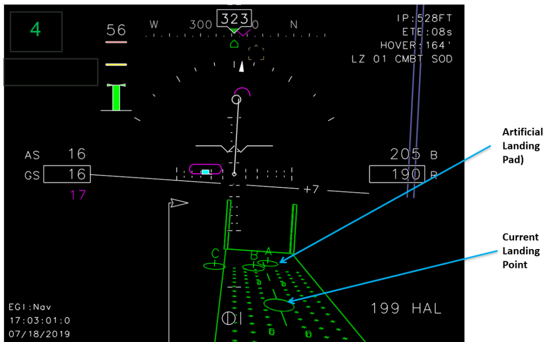
Figure B5. Right display: hover approach takeoff (HAT) page.
