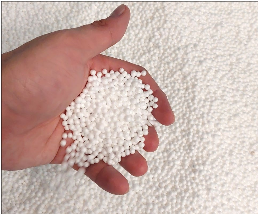
Figure 1. Expanded polystyrene pellets. Pellets were sprayed with industrial cleaner by the manufacturer to negate surface charge.
