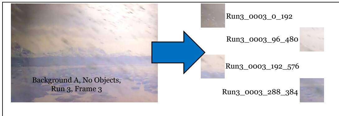
Figure 6. Conversion of individual frames ( left ) into 96 \times 96 px units ( right ).
