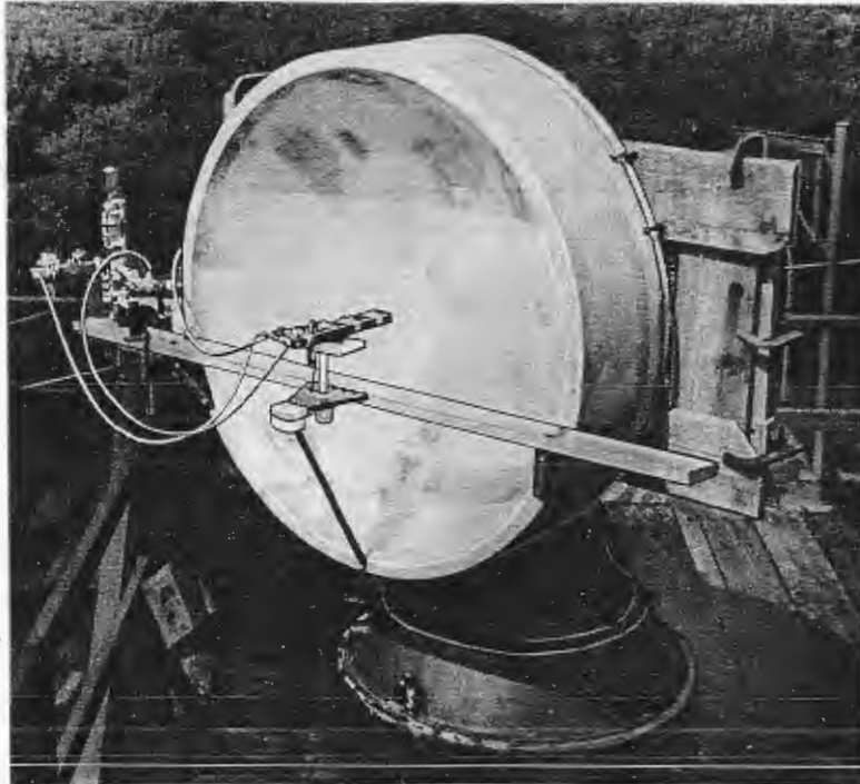
Figure 5 - Three-element primary feed mounted on spherical reflector
