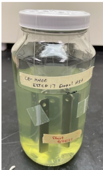
Figure C-1. Example Exposure Depicting the Material Coupons Suspended in Solution.
