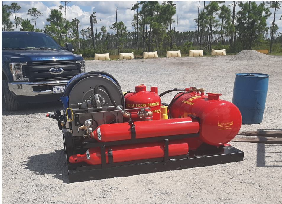
Figure 7. Dual-Agent CAF Skid for 315-ft 2 Fire Testing
