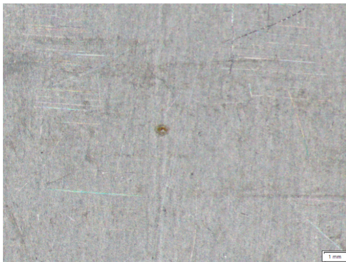
Figure C-19. Crevice Attack Observed on Stainless-steel Sample 28, Foam #13
