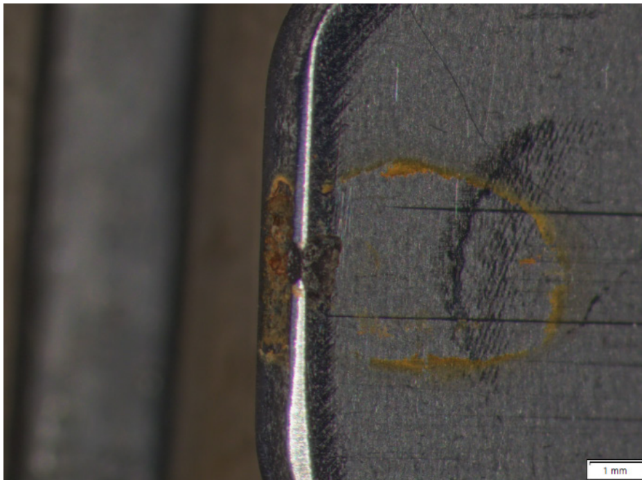
Figure C-18. Crevice Attack Observed on Stainless-steel Sample 29, Foam #11
