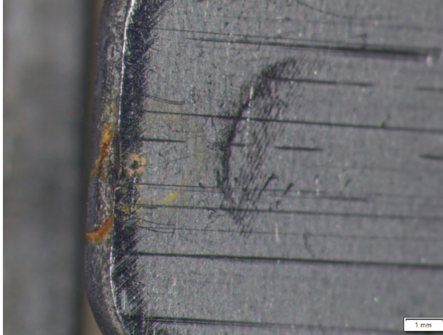
Figure C-17. Crevice Attack Observed on Stainless-steel Sample 23, Foam #11
