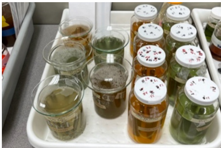
Figure C-2. AFFF Exposure Containment Cells –General and Localized Corrosion Rate Study.
