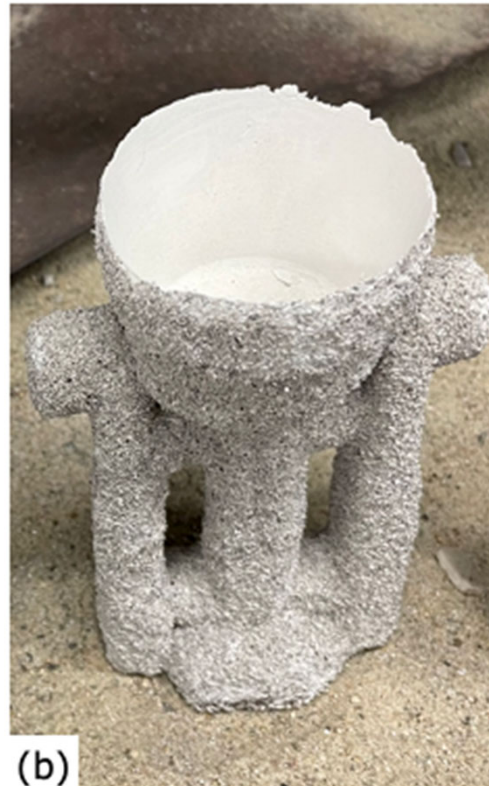
Ceramic shells after burnout (a) Part#12314649 casting tree assembly; (b) Part#12446263 casting tree assembly.
