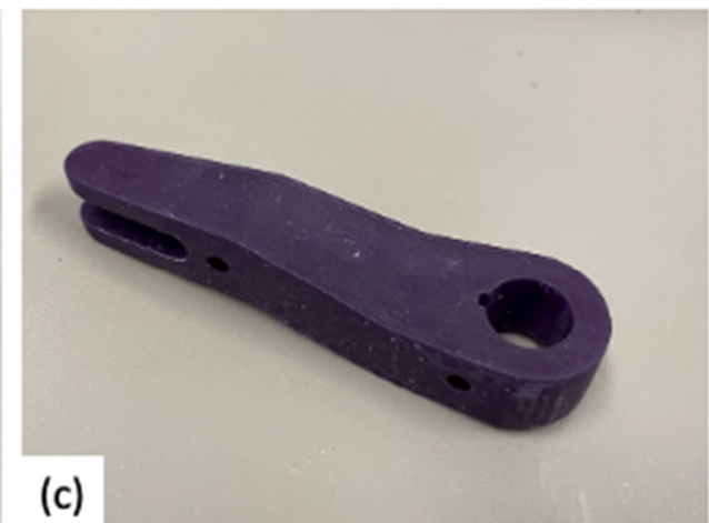
(a) Part #12314649 hollow pattern printed with 3D System Project 600HD; (b) Part#12446263 hollow pattern printed with Formlabs Form 2; (c) Part #154072 hollow pattern printed with Formlabs Form 2.
