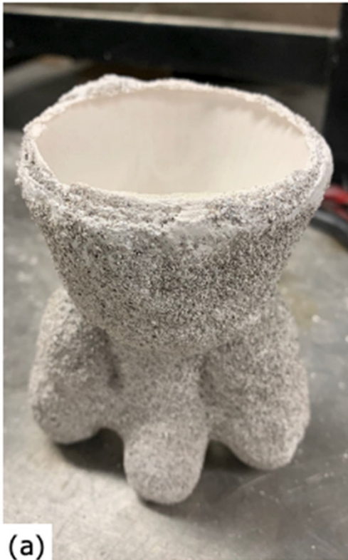
Ceramic shells after burnout (a) Part#12314649 casting tree assembly; (b) Part#12446263 casting tree assembly.
