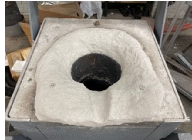
Mini-Melt furnace as built.
