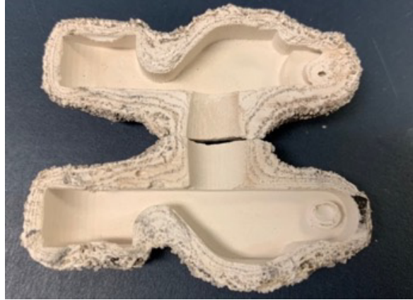
Figure 19. Ceramic shell (after burnout) is cut in half to carefully evaluate the internal surface.
