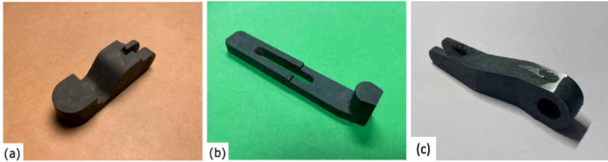
Figure 22. As-cast parts cut from casting tree (a) Part#12314649; (b) Part#12446263; (c) Part#154072.
