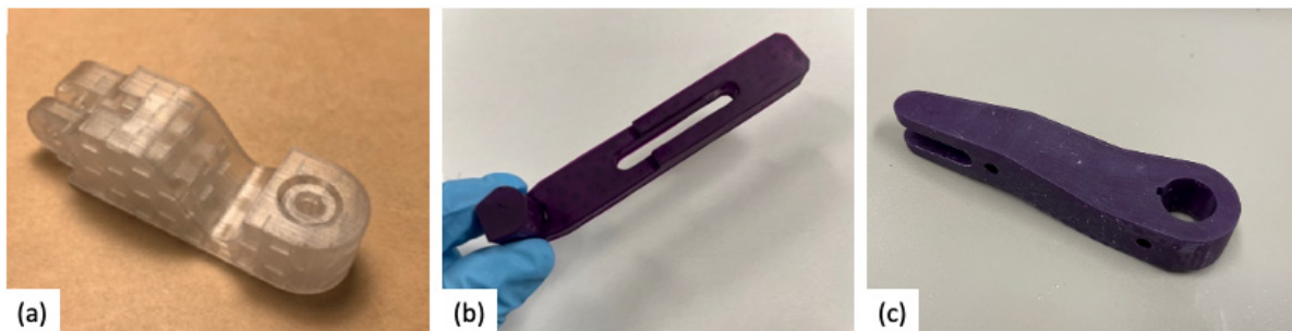
Figure 7. (a) Part #12314649 hollow pattern printed with 3D System Project 6000HD; (b) Part#12446263 hollow pattern printed with Formlabs Form 2; (c) Part #154072 hollow pattern printed with Formlabs Form 2.
