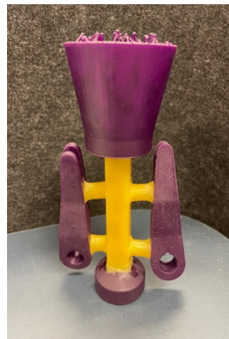
Figure 13. Casting tree assembly of Part #154072.
