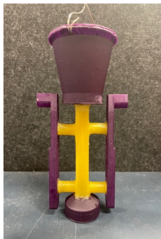
Figure 12. Casting tree assembly of Part #12446263.
