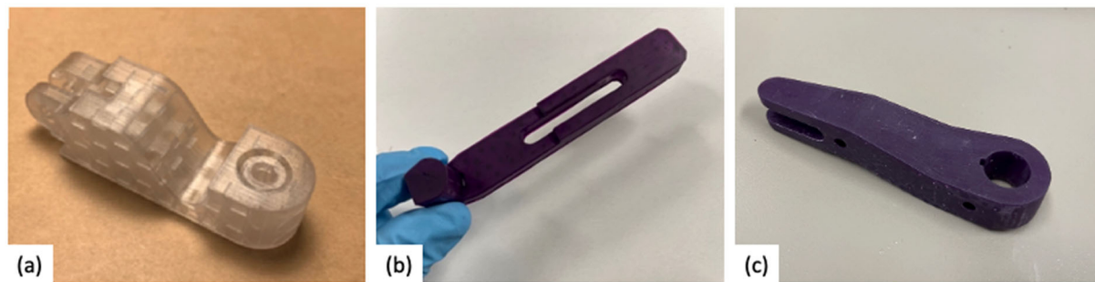
Figure 17 (a) Part 1 hollow pattern printed with 3D System Project 600HD; (b) Part 2 hollow pattern printed with Formlabs Form 2; (c) Part 3 hollow pattern printed with Formlabs Form 2.
