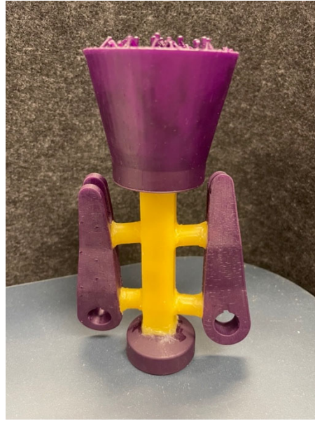
Figure 23 Casting tree assembly of Part 3.
