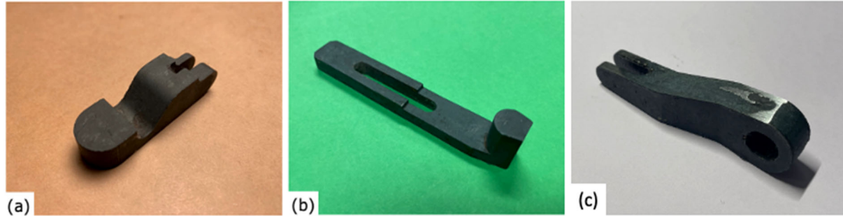
Figure 31 Parts cut from casting tree (a) Part 1; (b) Part 2; (c) Part 3.
