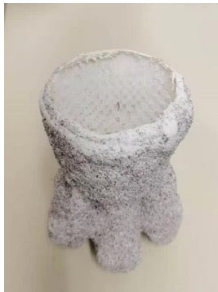
Figure 24 Completed ceramic shell before burnout.
