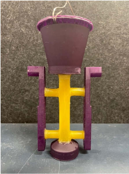
Figure 22 Casting tree assembly of Part 2.
