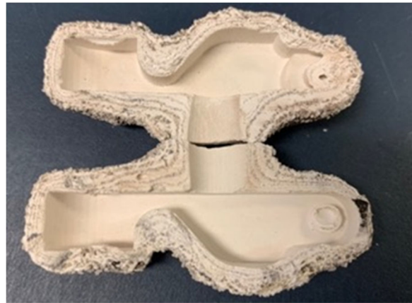
Figure 28 Cross-section view of ceramic shell after burnout.
