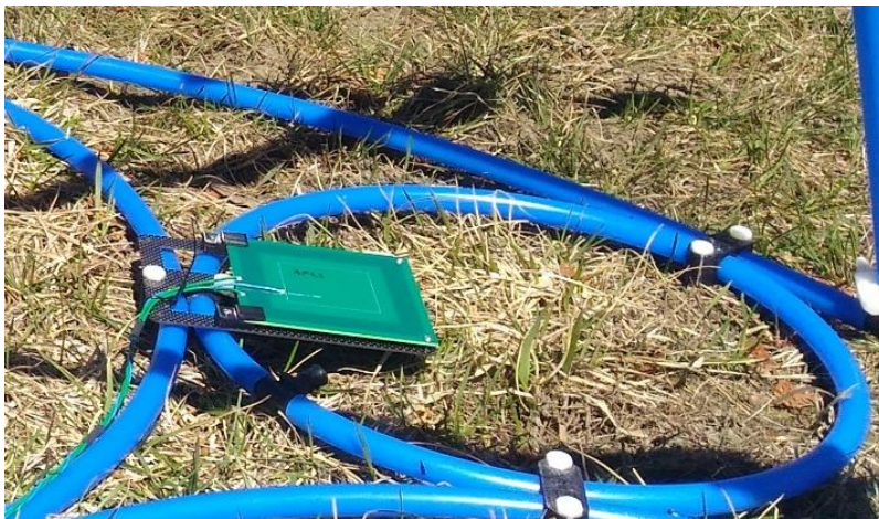
Figure 60. 10 Layer Rx PCB (green)
