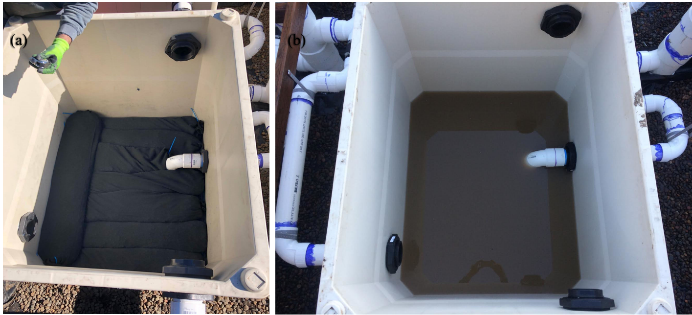
Figure 9: (a) Placement of Biochar and Aquagate (Rembind) in compost socks within macrobins; (b) Leaching of fines from LID before biochar is placed in macrobins.
