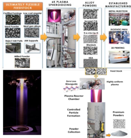
Plasma spheroidization process in the presence of hydrogen
