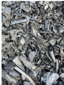
Auto-shred Aluminum Scrap (Twitch) 90-98 wt.% of mixed aluminum alloys
