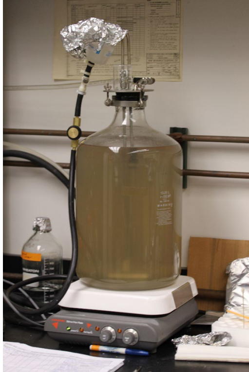
Figure 4.7. DF1 growth in glass bioreactor set up for testing the MBBR and FBR approaches to develop biofilms with DF1 on different substrates.
