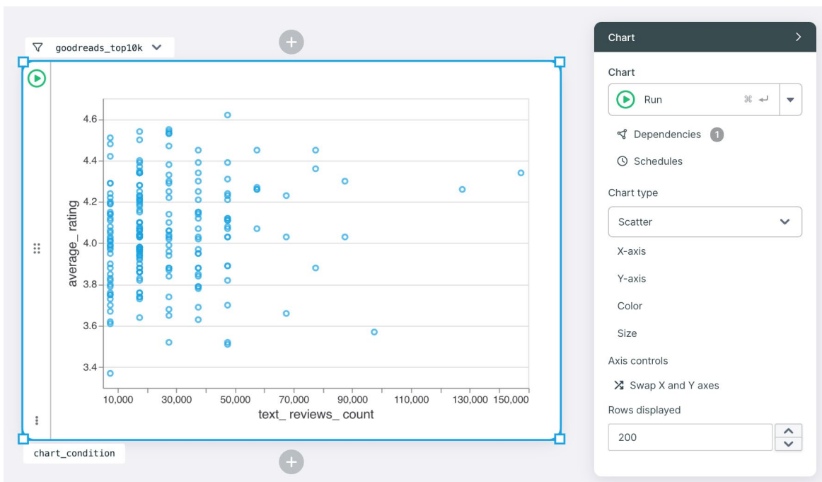
Figure 5: A no-code Chart cell that can be configured through the properties panel on the right. The UI is generated based on the cell manifest.
