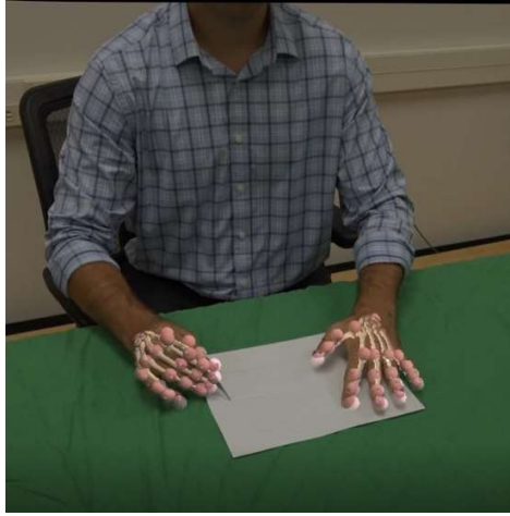
Figure 1545: Subject performing example task with inverse kinematics model from SwRI hand tracking system overlaid on video.
