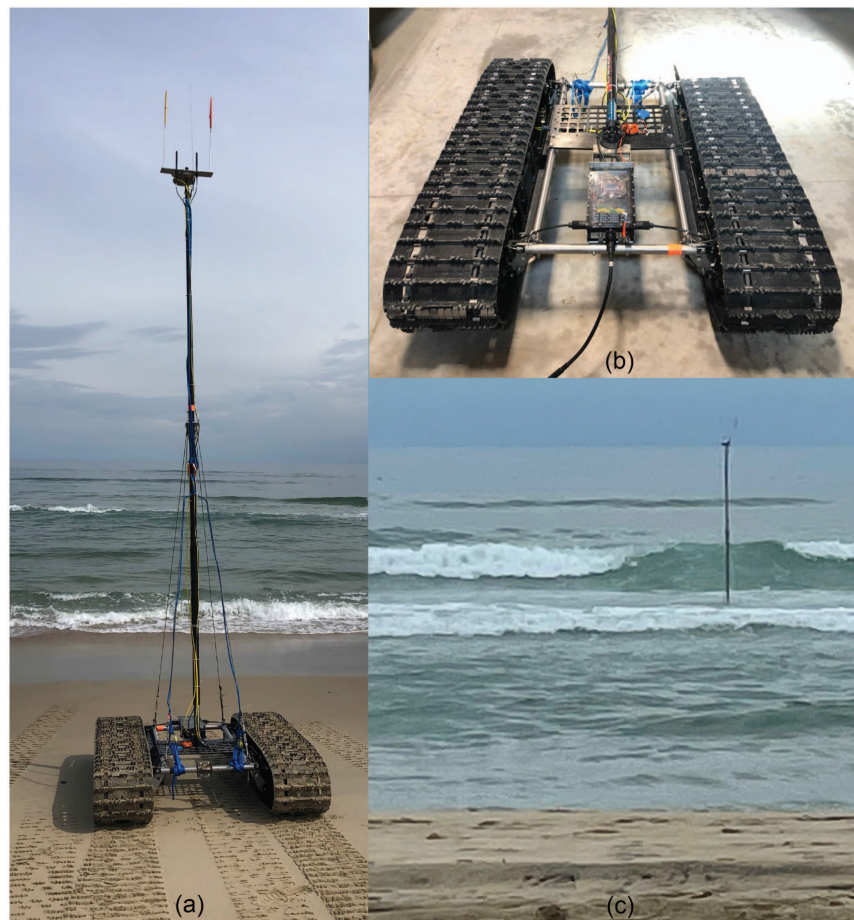
Fig. 1. (Color) (a) Crawler entering the water before repeatability test; (b) crawler charging in the garage with the vehicle mast laid down for storage; and (c) crawler traversing the surf at the FRF.
