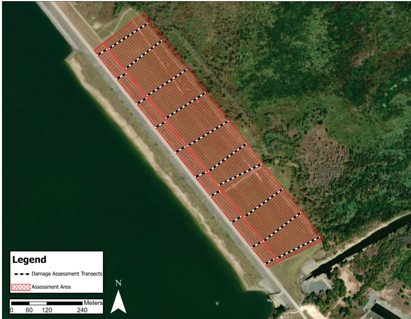
Figure 10. DAA-3 ( right of diagonal, large rectangle, levee flat ) and DAA-4 ( left of diagonal, thin rectangle, levee slope ) that were assessed as USACE infrastructure where feral swine damage had been identified by local staff at the Somerville Lake project, Texas. (Map image is the intellectual property of Esri and is used herein under license. Copyright © 2023 Esri and its licensors. All rights reserved. Map data: Maxar.)
