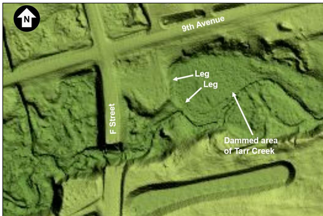
Figure 163. Lidar image showing the Tarr Creek dam structure. (Image from Wisconsin State Cartographer's Office. Modified by ERDC-CERL, 2023. Public domain.)
