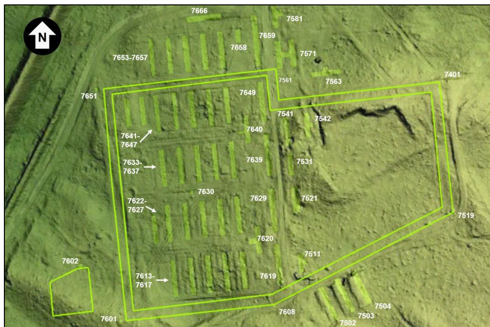
Figure 162. Lidar imagery of Compound A, including the footprints of former buildings and fences. (Image from Wisconsin State Cartographer's Office. Modified by ERDC-CERL, 2023. Public domain.)
