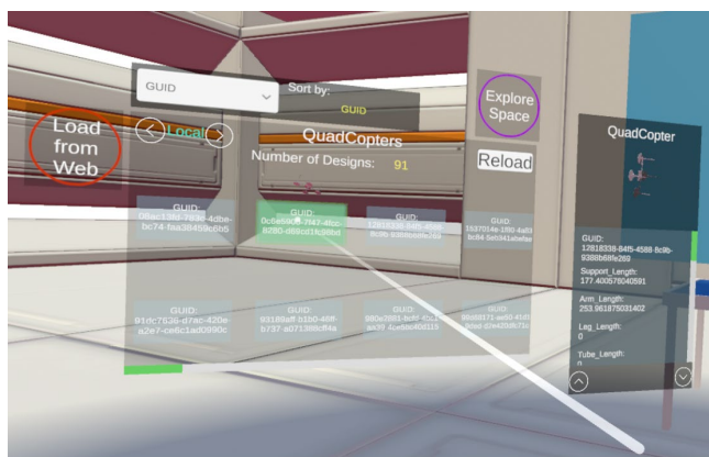
Figure 23 The main panel of the infinite shelf, with data loading function button on left, sliding design browser in the middle, and parameter visualizer on the right.
