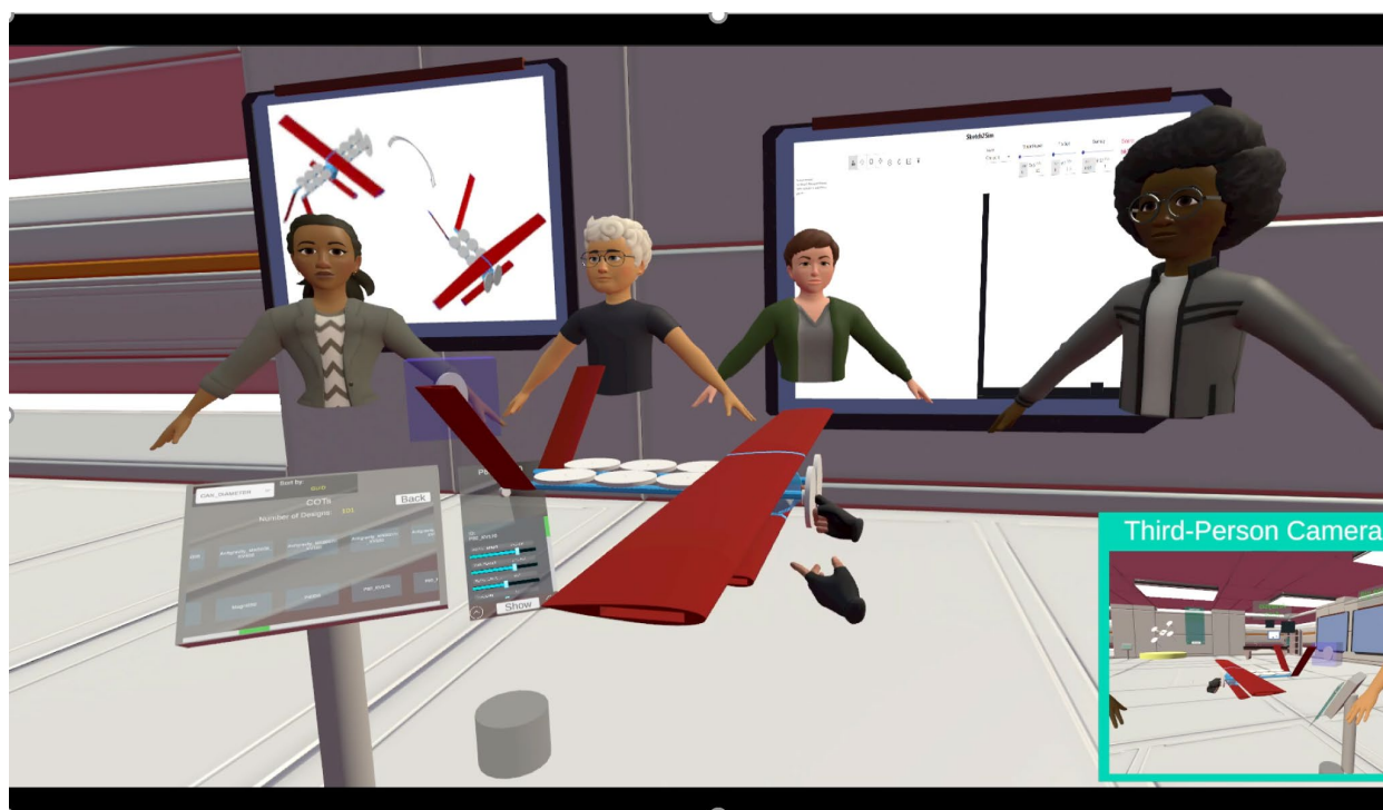
Figure 10 Design composition in VR. Multiple users can participate. The inset in the lower right shows a 3 rd person view of the design process from the room.
