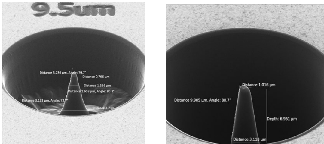
Fig. 3. Electron microscope images of cone structures that were fabricated from silicon aiming for the dimensions that modeled in Figure 2.
