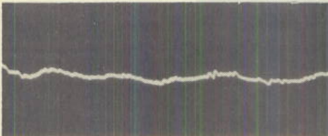
Figure 3.10. Echo signal from submarine hull
